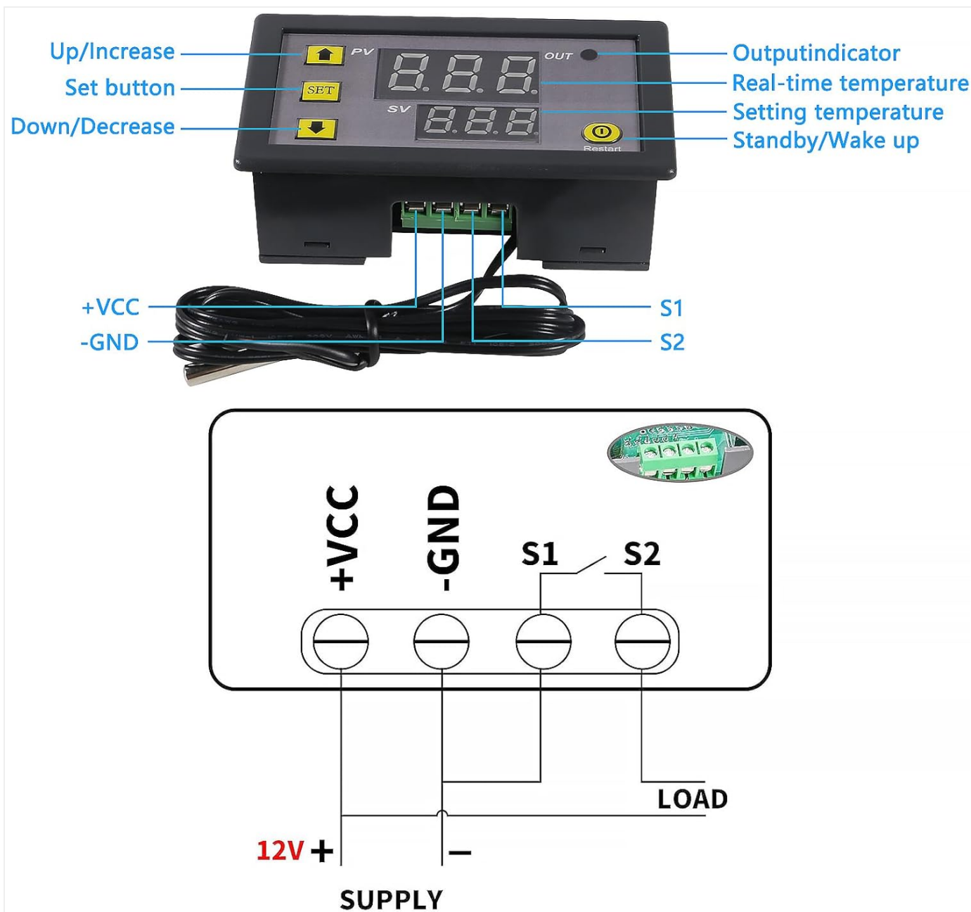
Figure 2: Detailed wiring diagram for the W3230 controller. It illustrates connections for the power supply (+VCC, -GND) and the load (S1, S2) to the relay output.
