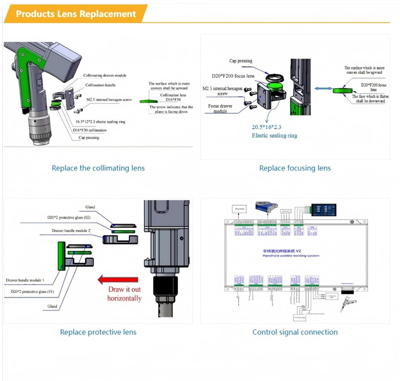
Figure 4: Diagram illustrating the control signal connections for the handheld welding system. (Note: This image also contains lens replacement diagrams, but the relevant part for setup is the control signal connection.)
