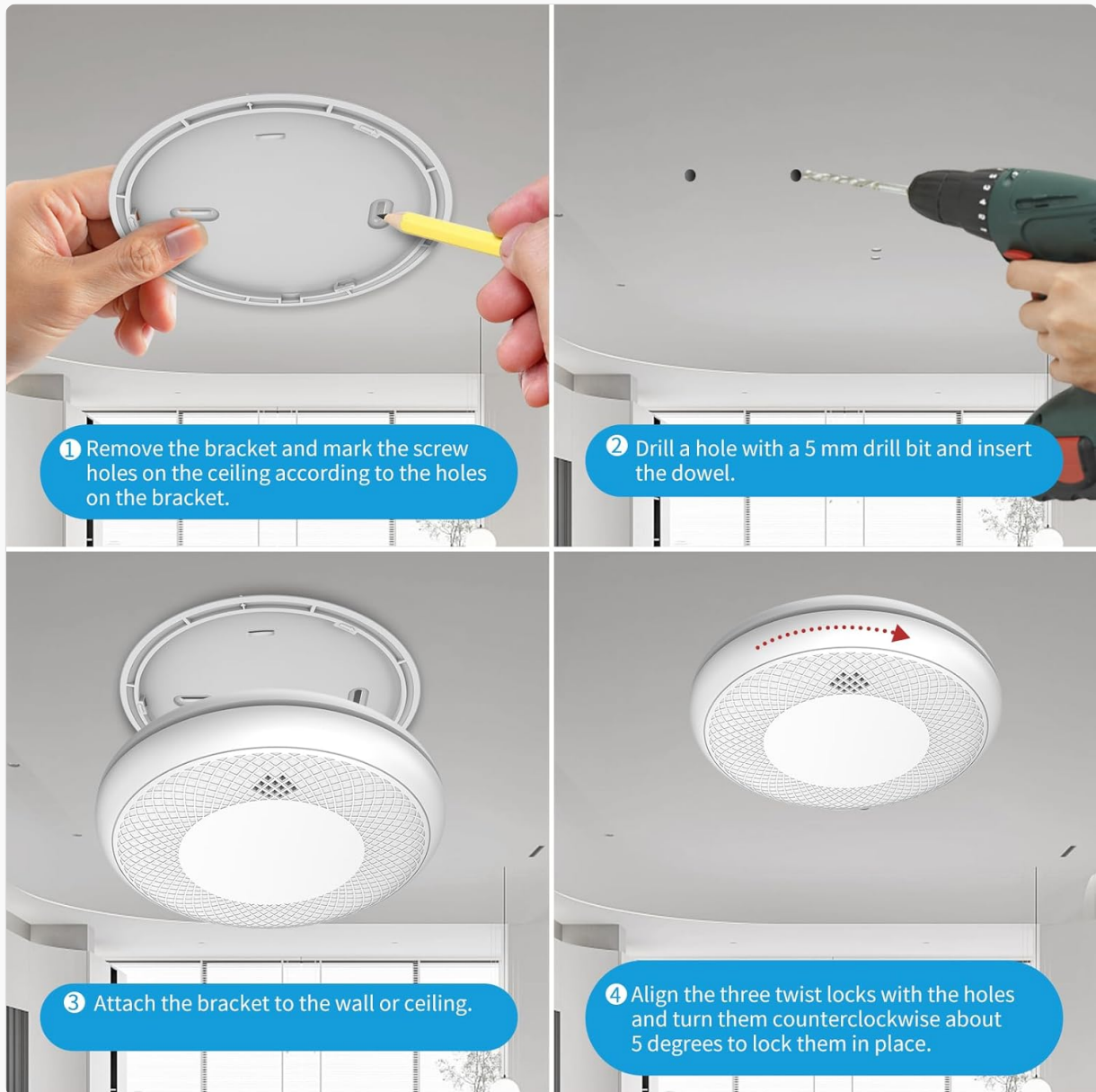
Image: Step-by-step visual guide for screw-based installation of the smoke detector.
