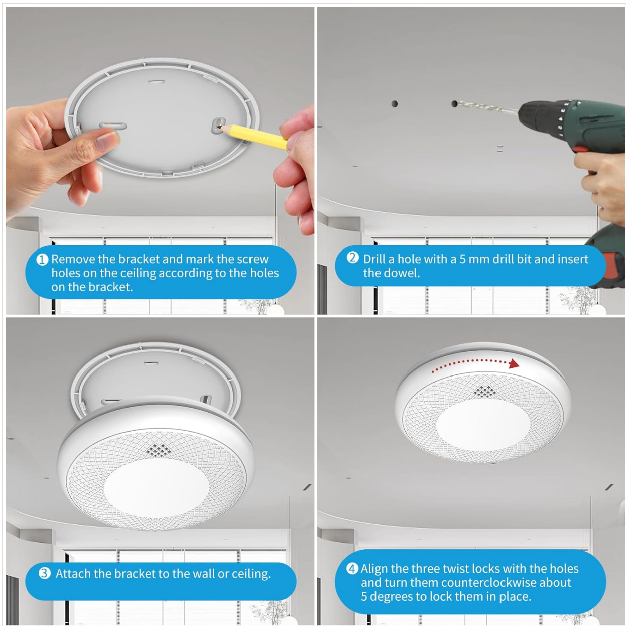
A visual guide demonstrating the four steps for installing the smoke detector: marking screw holes, drilling and inserting a dowel, attaching the bracket, and twisting the detector onto the bracket.
