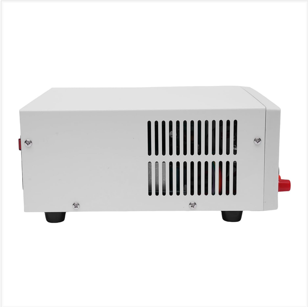
Figure 4.2: Side view of the EBC-A10H, highlighting the air vents for heat dissipation.
