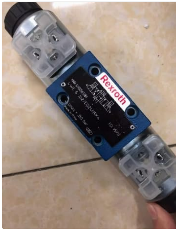
Figure 1: Rexroth Hydraulic Electromagnetic Directional Valve, Model 4WE6J6X-EG24N9K4. This image displays the Rexroth hydraulic electromagnetic directional valve, model 4WE6J6X-EG24N9K4. The valve features a blue central body with the 'Rexroth' logo and model number '4WE 6 J62/EG24N9K4' clearly visible. It also indicates a maximum pressure of 350 bar. Transparent plastic covers are visible on both ends, protecting the electrical connections.
