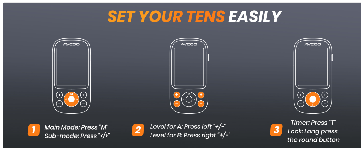
Image 6.1: Step-by-step guide for setting modes, levels, timer, and screen lock on the AVCOO TENS EMS Unit.
