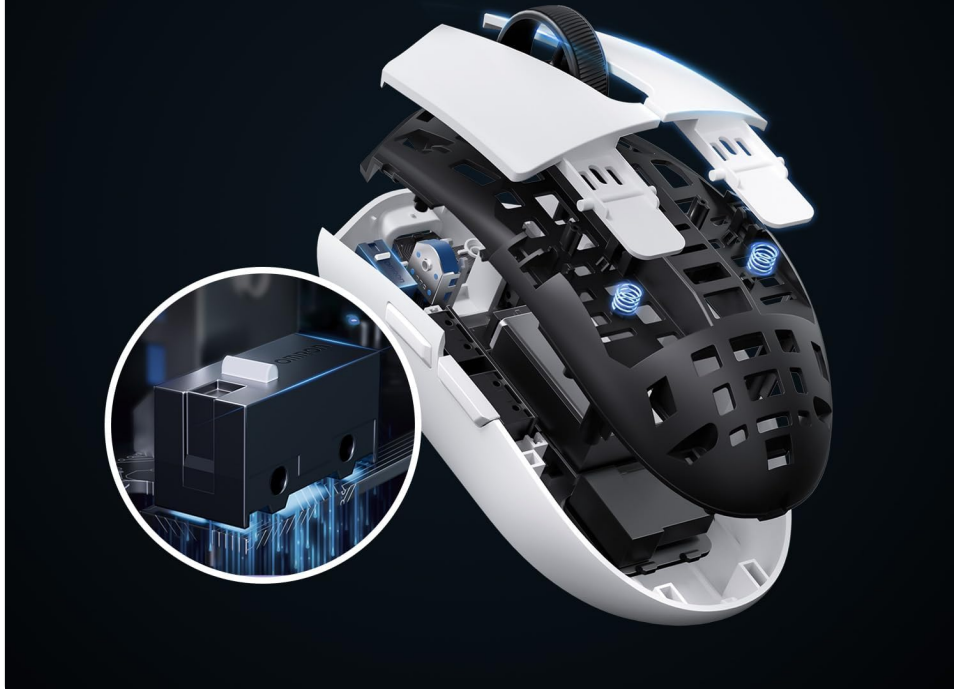
Figure 7: Internal view highlighting the Independent Button Pressure System for consistent click feel.
