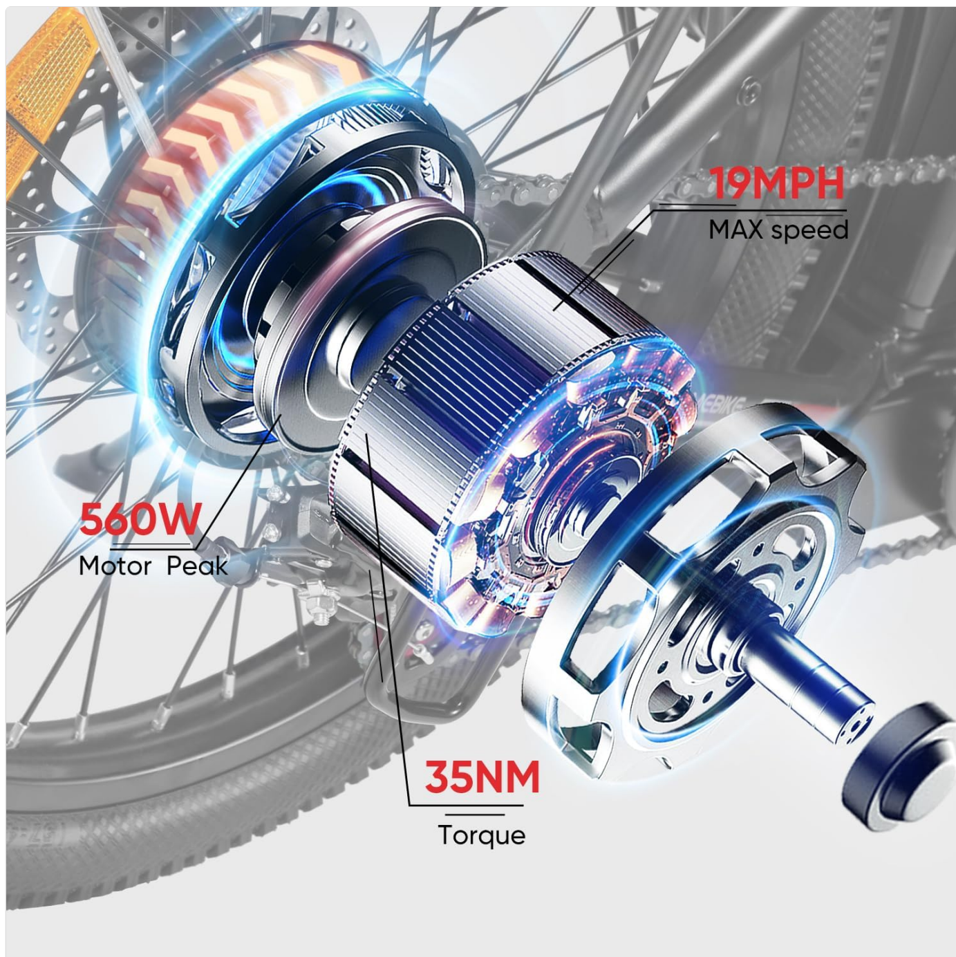
Image: An exploded view diagram of the SAMEBIKE electric bike's 560W peak motor and rear disc brake, illustrating the internal components and braking mechanism.
