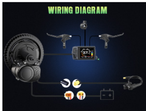
Image: Simplified wiring diagram illustrating connections between the motor, display, brake levers, throttle, speed sensor, and battery.
