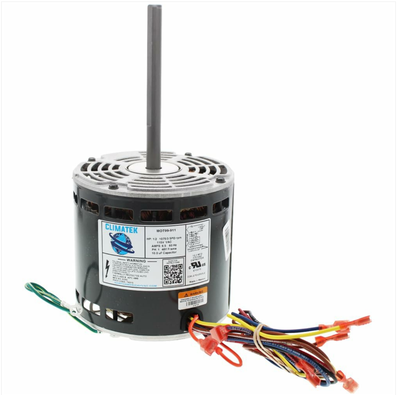
Figure 1: ClimaTek Furnace Blower Motor (Model MOT99-911). This image displays the main body of the motor, its central shaft, and the attached electrical wiring. The product label is visible, indicating key specifications such as 1/2 HP, 1075/3 SPD rpm, 115V VAC, 6.5 AMPS, 60 Hz, PH 1, 48Y Frame, and a 10.0 uF Capacitor requirement.
