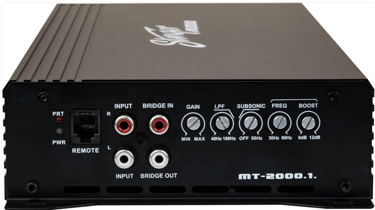
Image: Rear view of the STINGER MT-2000.1 amplifier showing the control panel. Labels include PRT (Protection Indicator), PWR (Power Indicator), REMOTE port (for bass knob), INPUT RCA (L/R), BRIDGE IN RCA, GAIN knob (Min/Max), LPF knob (40Hz-180Hz), SUBSONIC knob (OFF/50Hz), FREQ knob (30Hz/80Hz), BOOST knob (0dB/12dB), and INPUT BRIDGE OUT RCA.
