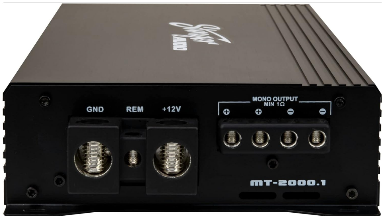
Image: Rear view of the STINGER MT-2000.1 amplifier showing the power and speaker terminals. Labels include GND (Ground), REM (Remote Turn-on), +12V (Power), and MONO OUTPUT MIN 1 Ohm speaker terminals (+ and -).
