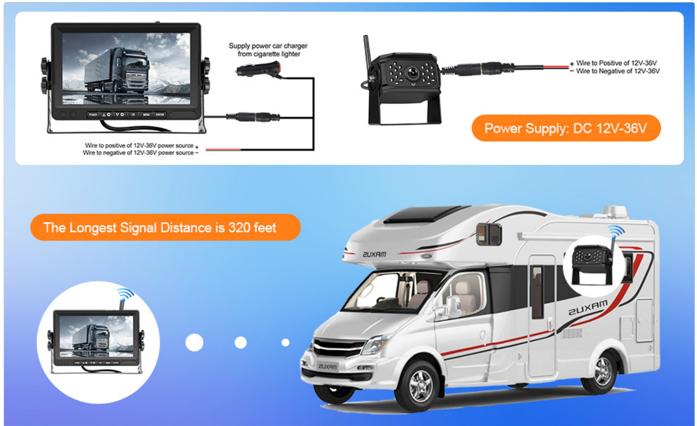
Figure 2: Connection Diagram. This image shows how to connect the monitor and camera, including power supply options and antenna placement. The camera connects to a 12V-36V power source, and the monitor can be powered via a cigarette lighter or direct wiring.
