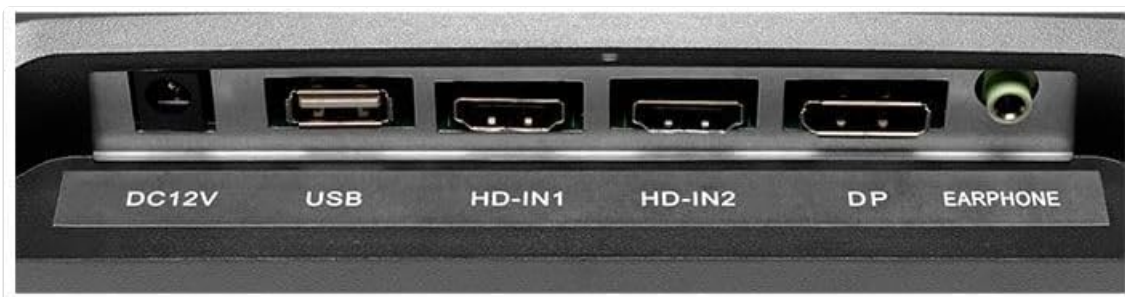
Image: Rear view of the monitor's connectivity panel, showing DC12V power input, USB port, two HDMI inputs (HD-IN1, HD-IN2), a DisplayPort input (DP), and an earphone jack.
