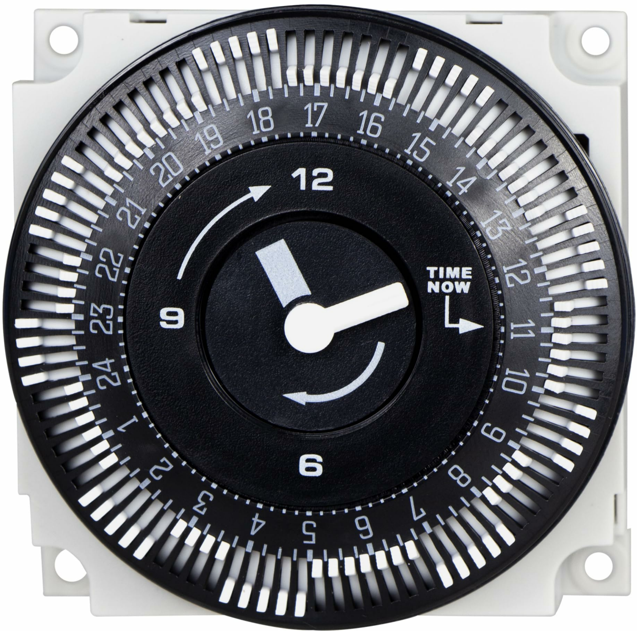
Figure 1: Front View of the KERDE TJ01-G Timer. This image displays the timer's front face, featuring a black dial with white numbers indicating hours (1-24) and a central clock-like mechanism with a "TIME NOW" arrow. Around the dial, numerous white pins are visible, which are used to set the on/off intervals.
