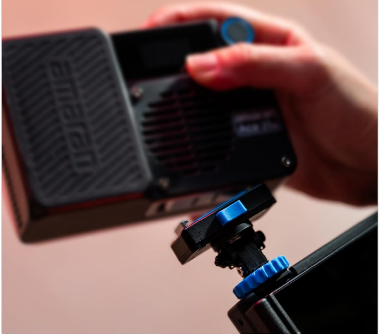
Close-up image showing the Amaran Ace Lock quick mount bayonet system for one-second removal and installation.
