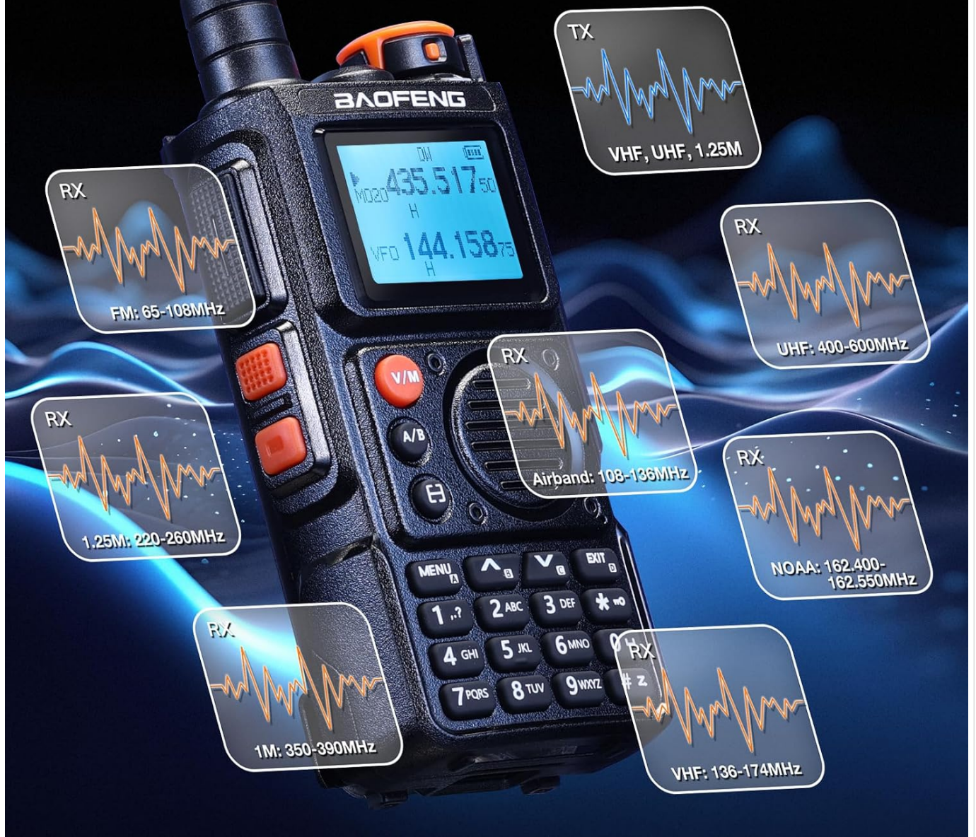
Image: Visual representation of the multi-band transmit and receive capabilities of the BAOFENG K6 across various frequency ranges.
