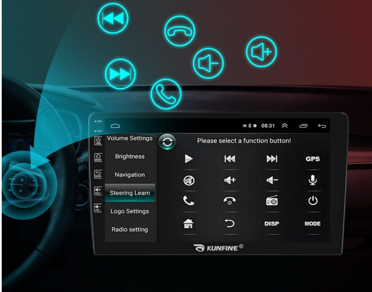
Figure 10: Steering Wheel Control. The head unit displays a menu for learning and mapping steering wheel control functions, with icons representing various commands.
