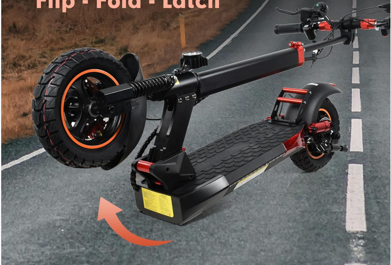
Figure 3: Quick folding mechanism for portability.
