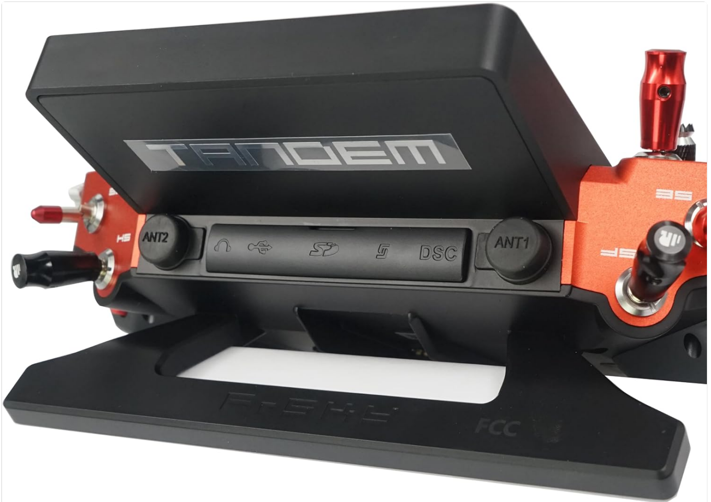
Figure 4.1: Top view of the FrSky TANDEM X20 PRO AW transmitter, highlighting the antenna ports (ANT1, ANT2), headphone jack, USB-C port, and DSC port. This view is crucial for understanding connectivity options.
