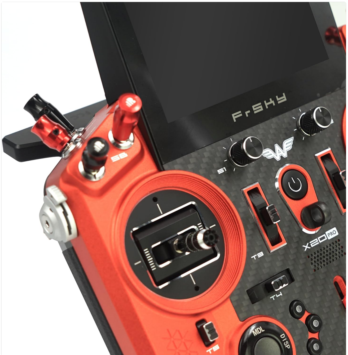
Figure 5.1: Detailed view of the FrSky TANDEM X20 PRO AW's high-precision Hall-Sensor MC20R gimbals and surrounding switches. This image emphasizes the ergonomic design and the quality of the control sticks, essential for fine motor control of UAVs.
