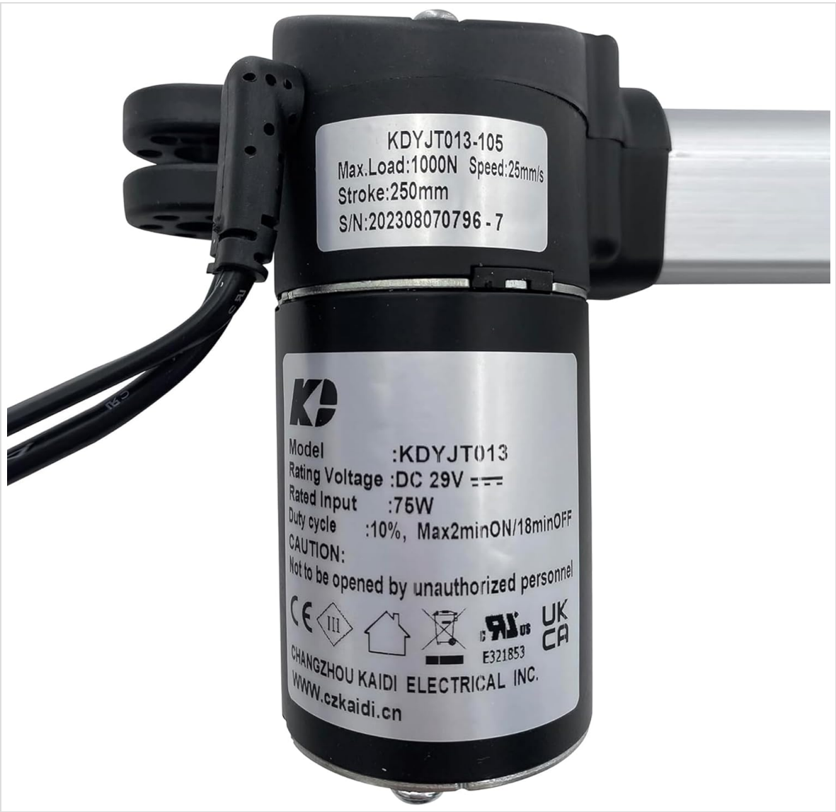
Image: Close-up view of the Kaidi KDYJT013-105 linear actuator motor label, showing model number, maximum load, stroke, speed, rating voltage (DC 29V), rated input (75W), and duty cycle (10%, Max 2min ON/18min OFF).
