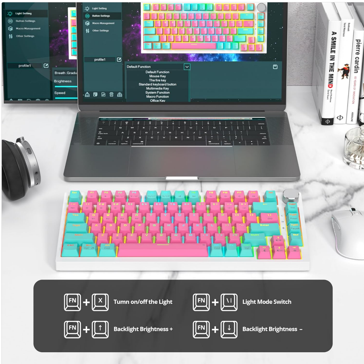
Figure 4.2: Keyboard RGB and software customization. This image shows the keyboard connected to a laptop, displaying software for customizing RGB lighting and key functions. It also highlights key combinations for backlight control: Fn+X to turn on/off the light, Fn+\ to switch light modes, Fn+Up Arrow to increase backlight brightness, and Fn+Down Arrow to decrease backlight brightness.
