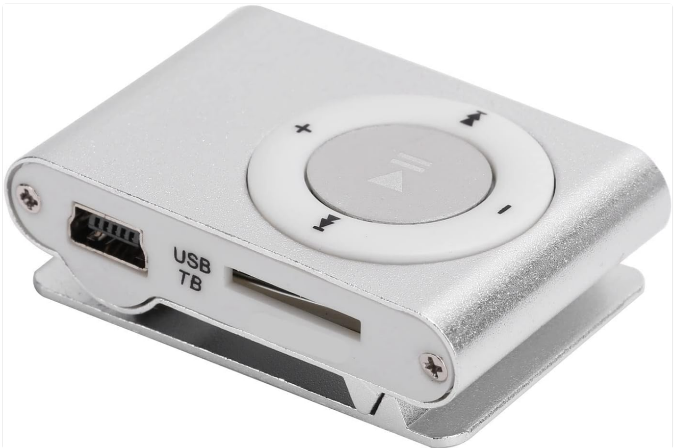
Image: Side view of the MP3 player, illustrating the USB charging/data port and the MicroSD card expansion slot.
