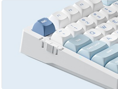
Figure 3.1: Location of the mode switch on the side of the keyboard for selecting connection type.
