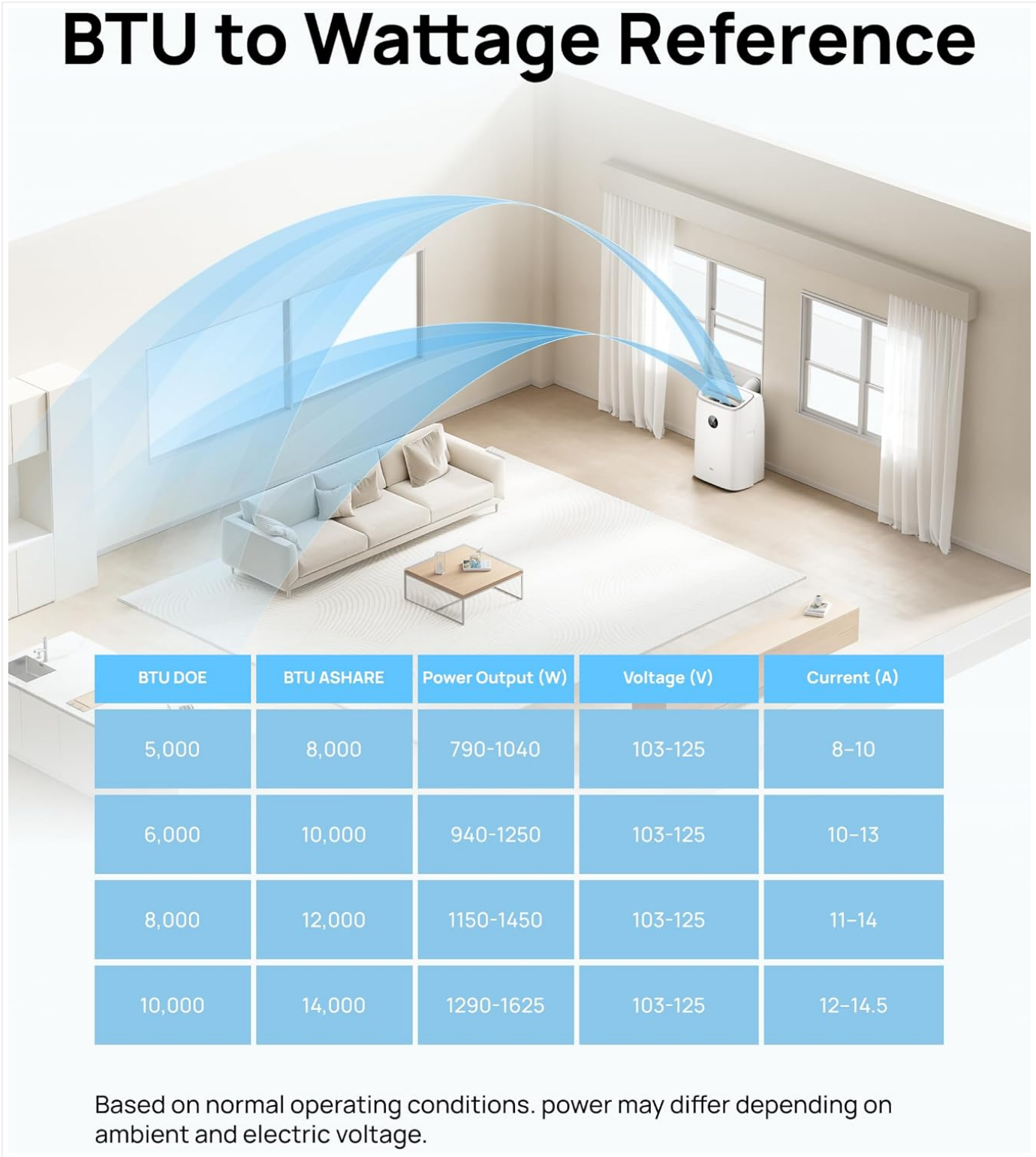
Figure 9.2: Power Consumption Reference. This table details the power output (Wattage), voltage, and current draw for different BTU ratings (DOE and ASHRAE). For the 12,000 BTU ASHRAE (8,000 BTU DOE) model, the power output is typically 1150-1450W, with a voltage of 103-125V and current of 11-14A. Note that power may differ depending on ambient and electric voltage.
