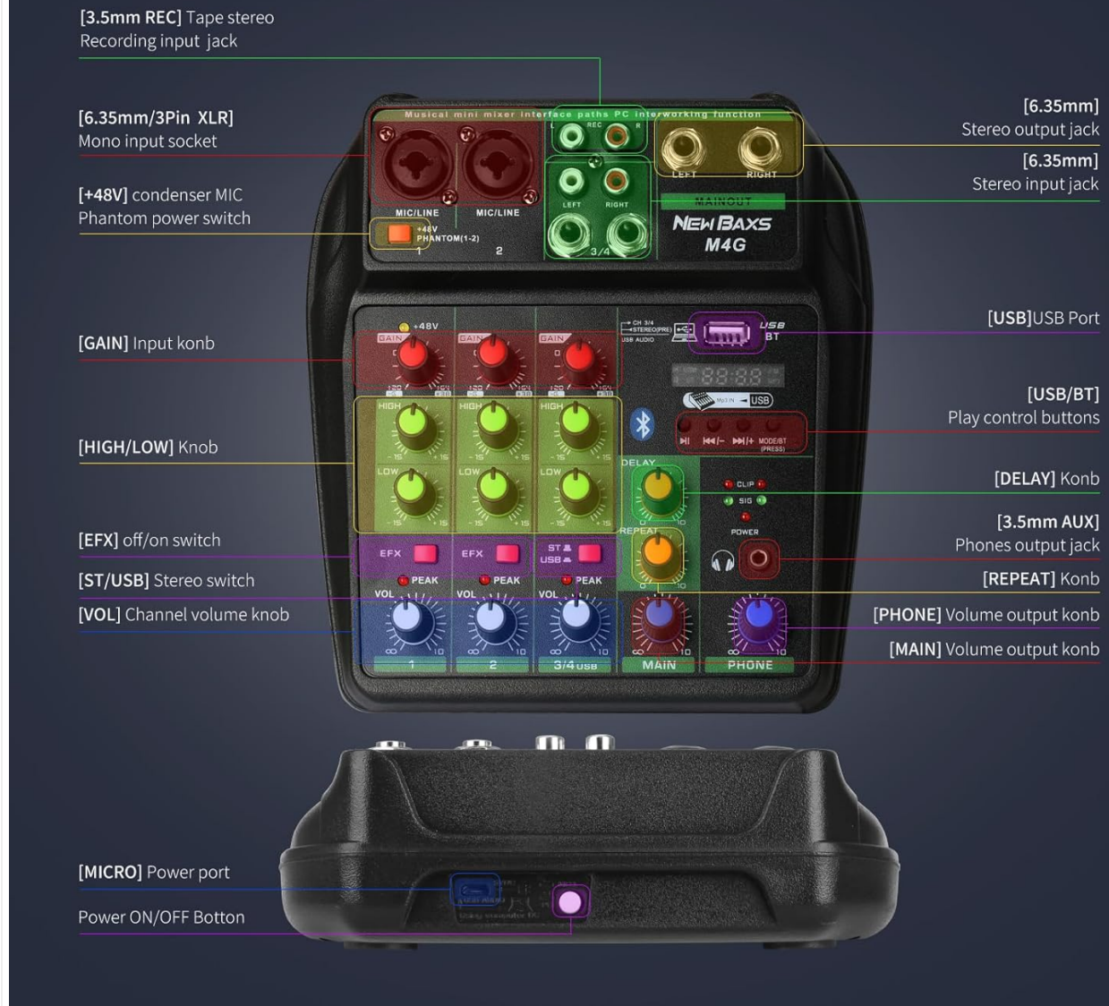
Figure 8: Labeled controls of the NEW BAXS M4G Audio Mixer.
