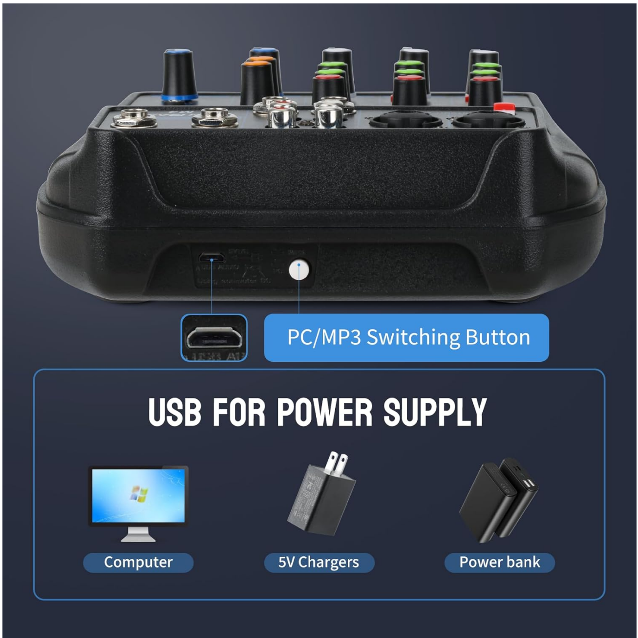
Figure 3: USB power supply options for the mixer.
