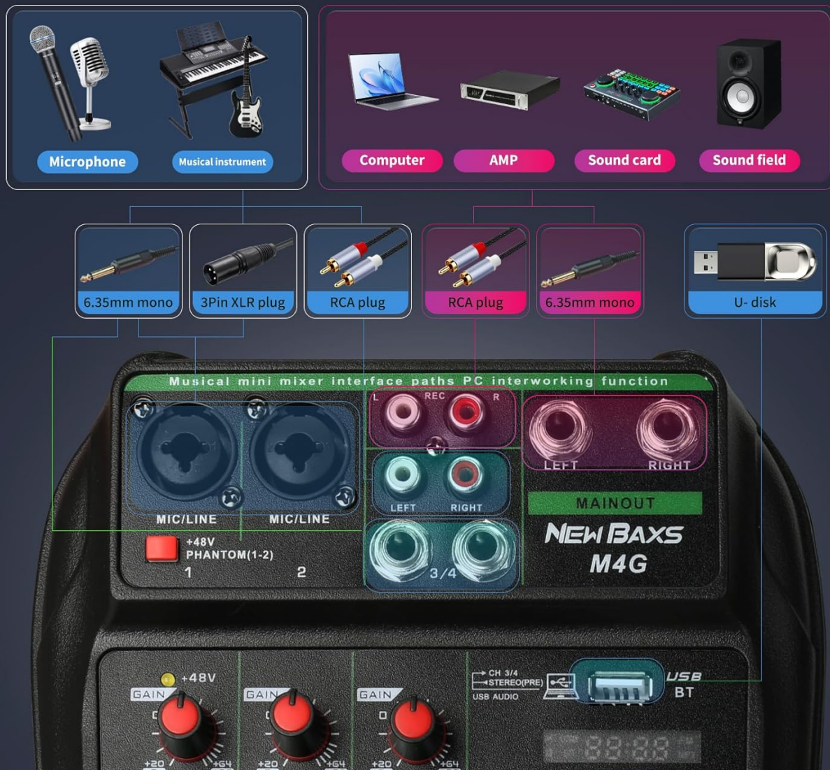
Figure 4: Overview of supported device connections.
