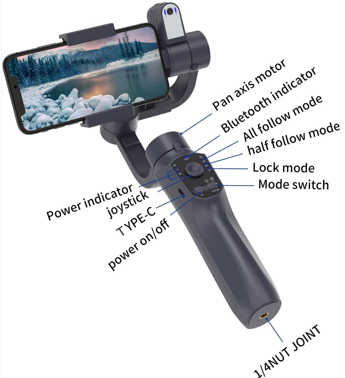
Image: Diagram illustrating the various controls on the Desional 3-Axis Gimbal Stabilizer, including the joystick, power indicator, Type-C port, power button, mode switch, and 1/4 nut joint.
