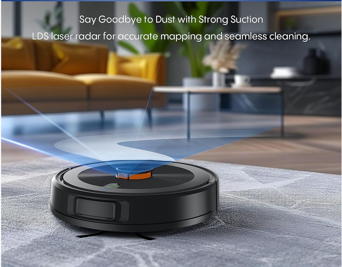
Image 4.1: The Bagotte BL20 utilizing its LiDAR navigation system to map and clean a room.
