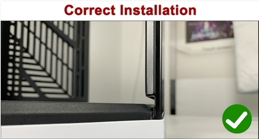
Correct installation: Monitor fully inserted into the side panel.
