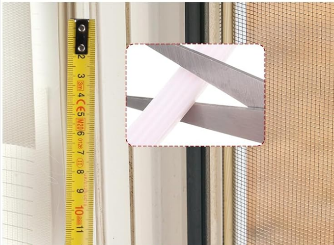
Measure and Trim any excess length for a custom fit.
