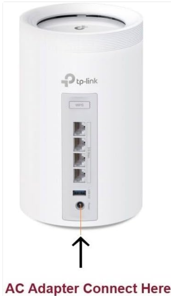
Figure 3: Example of connecting the AC adapter to a compatible TP-Link Deco device. The arrow indicates the power input port.
