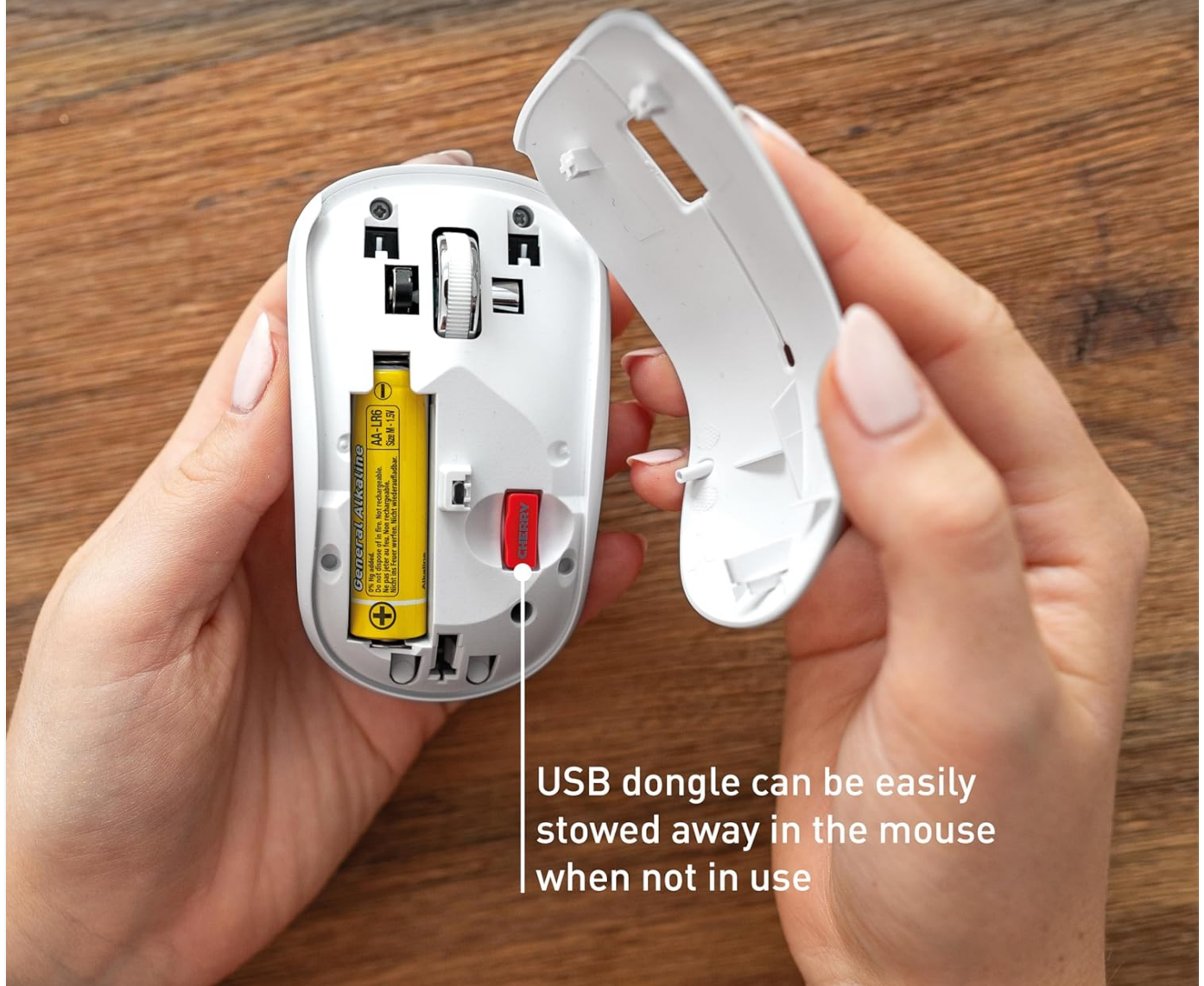
Image: The internal compartment of the Cherry MW 2200 mouse, revealing the AA battery slot and the dedicated storage for the Nano USB dongle. This design ensures the dongle is secure when not in use.
