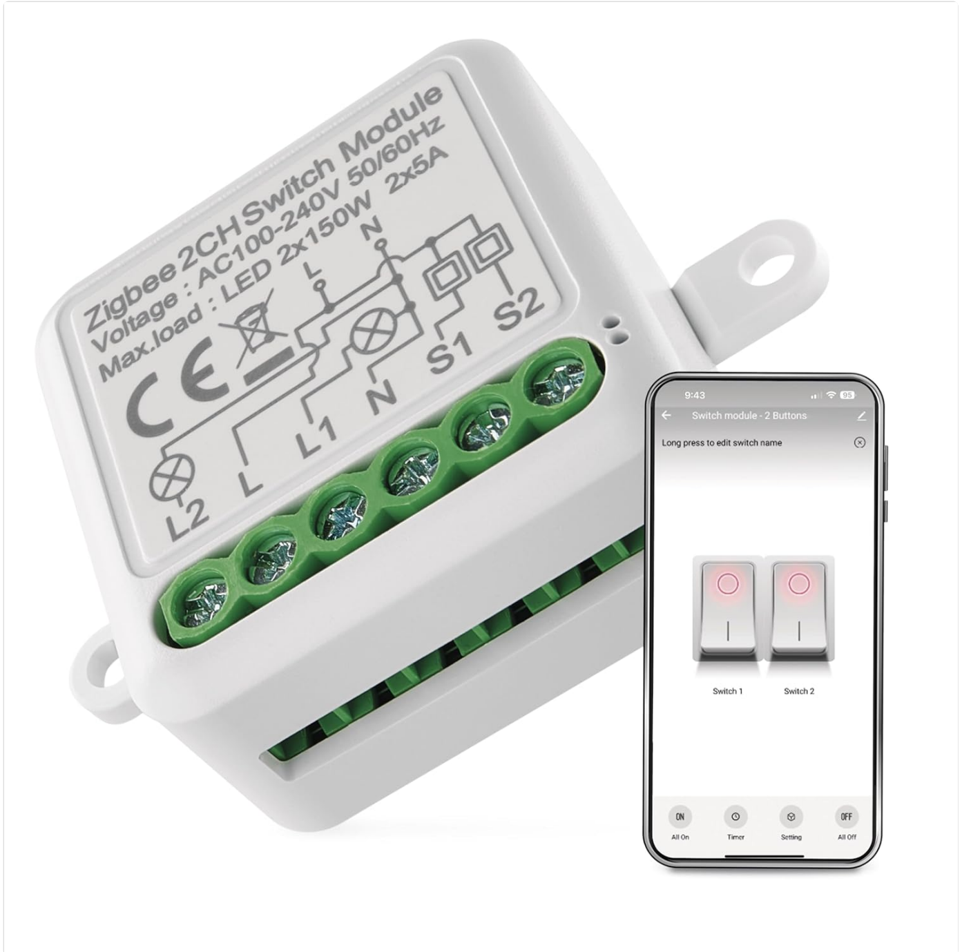
Figure 5.1: Module Wiring and App Control Example
