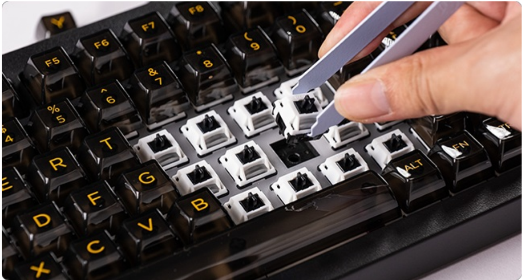
Image: A hand using a tool to remove a mechanical switch from the keyboard, demonstrating the hot-swappable feature.
