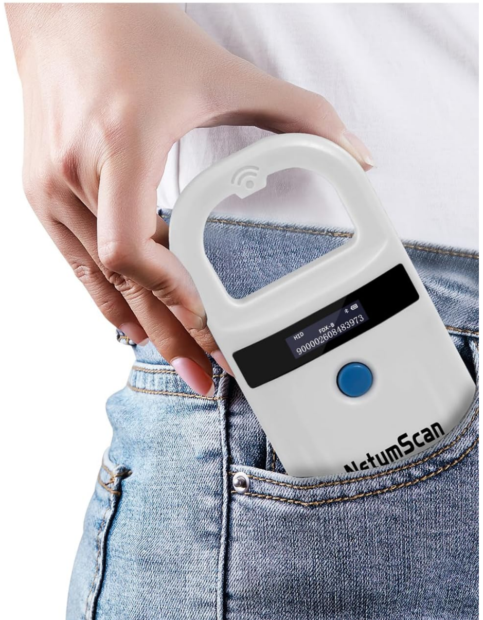
Image 2.1: The NetumScan DJ-180C device shown with its dimensions (135mm/5.3in length, 53mm/2.3in width) and weight (46g/1.6oz), demonstrating its compact size and portability, fitting easily into a pocket.
