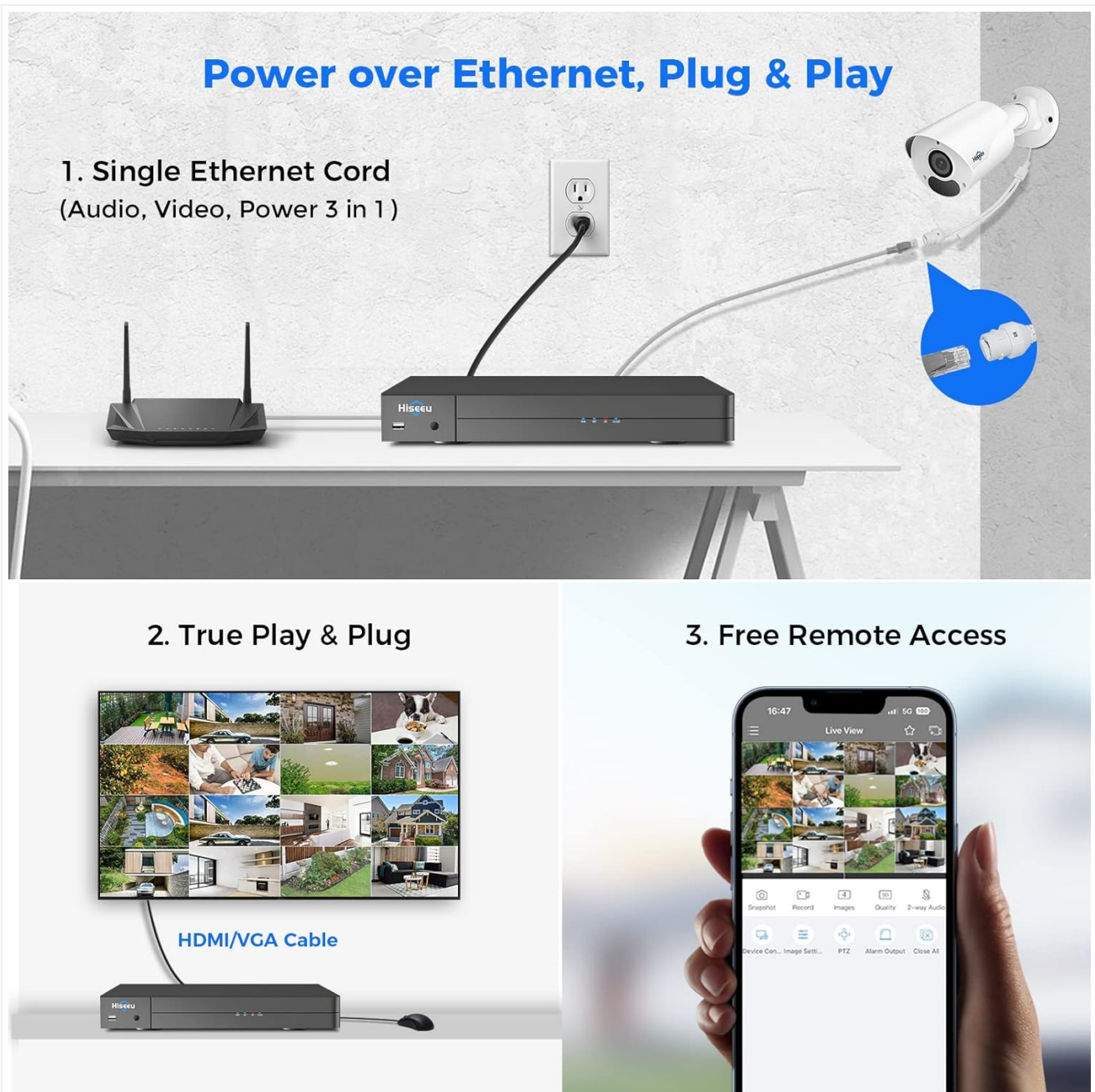
Figure 2.1: NVR Connection Diagram
