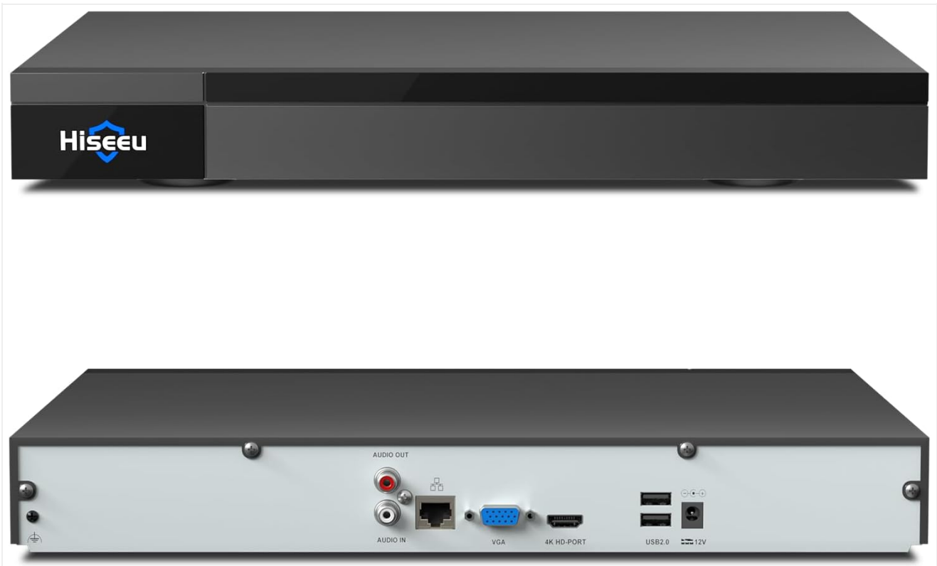
Figure 1.1: Hiseeu 4K 32 Channel PoE NVR - Front and Rear Panels
