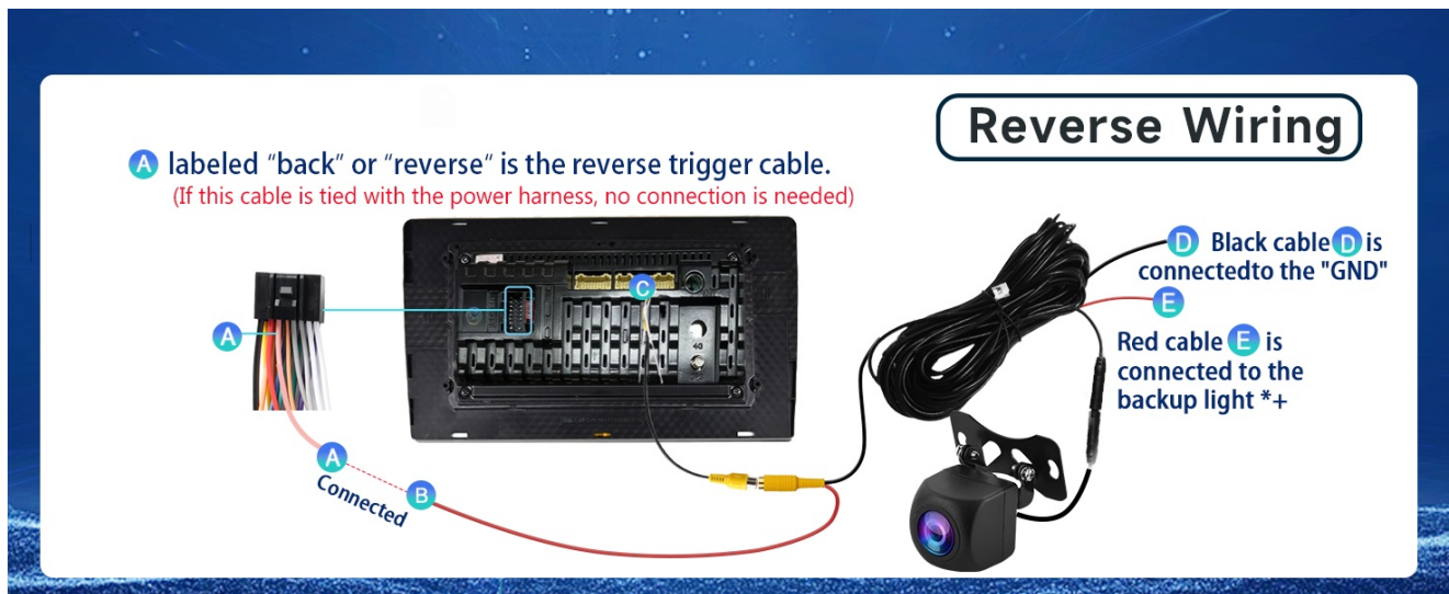
Image 4.2: A detailed diagram showing the connections for the reverse camera, including the video signal cable and the power/trigger wires.
