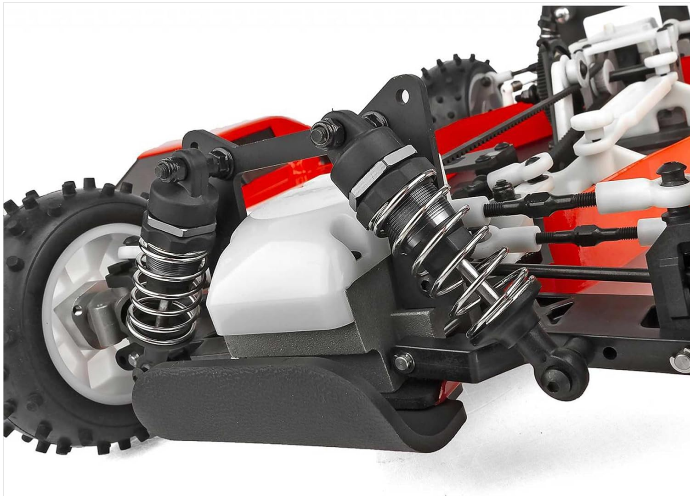
Image 4.1: Close-up of the front suspension and threaded shocks, illustrating components that require regular inspection and maintenance.
