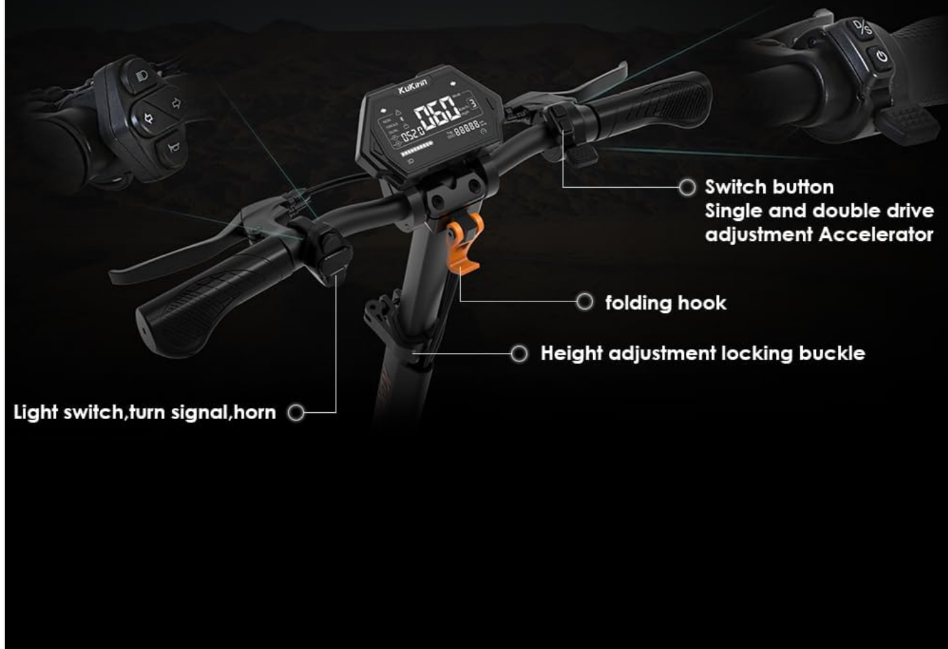
Figure 2: Close-up of the handlebar control area, showing the display, switch button, folding hook, and height adjustment locking buckle.
