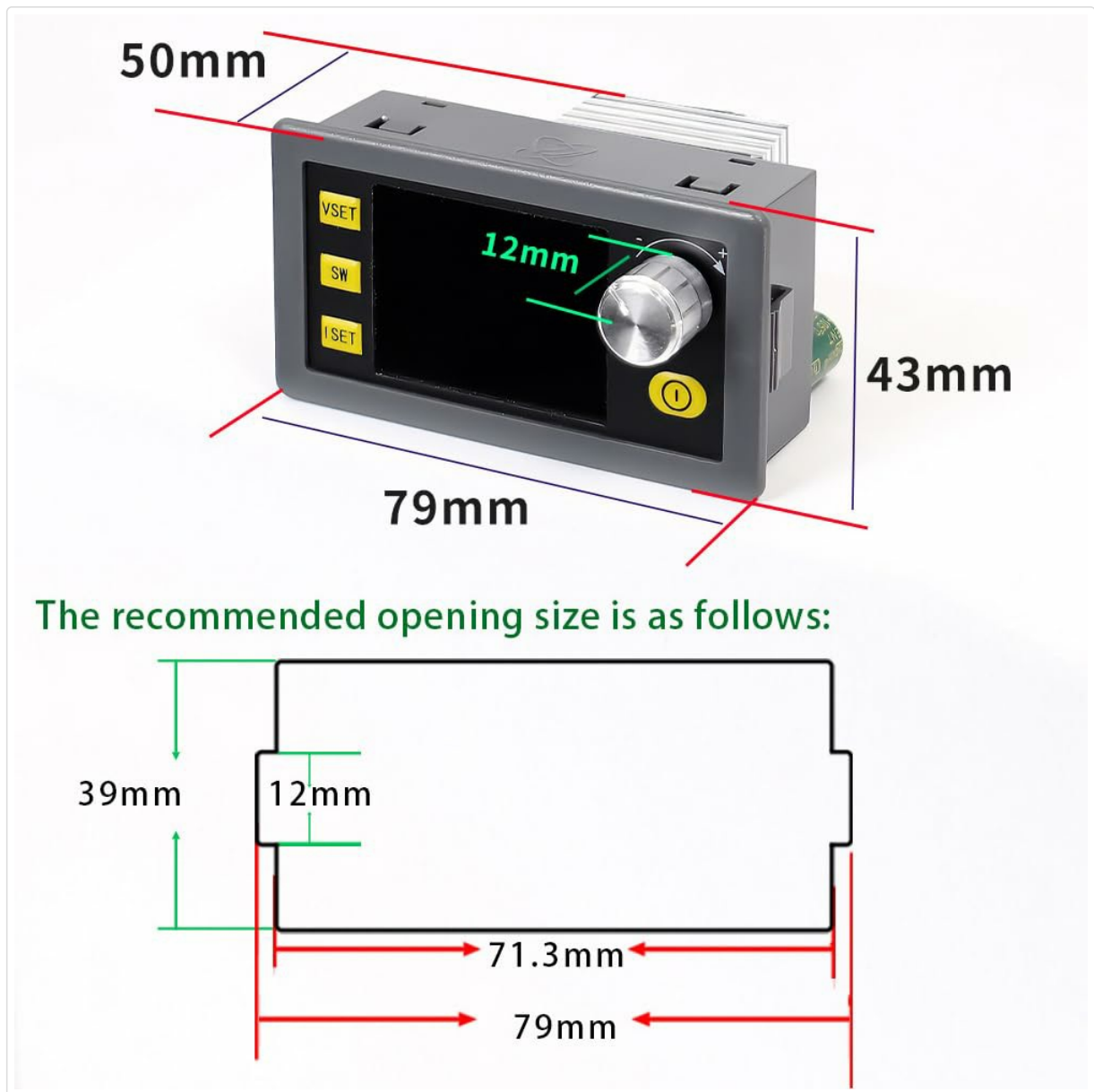
Figure 2: Physical dimensions of the XY-SK60 module and recommended panel cutout.
