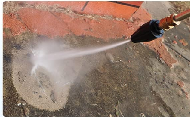
Image: Diagram illustrating the rotating conical spray pattern of the turbo nozzle, highlighting its effectiveness for fast and powerful cleaning.
