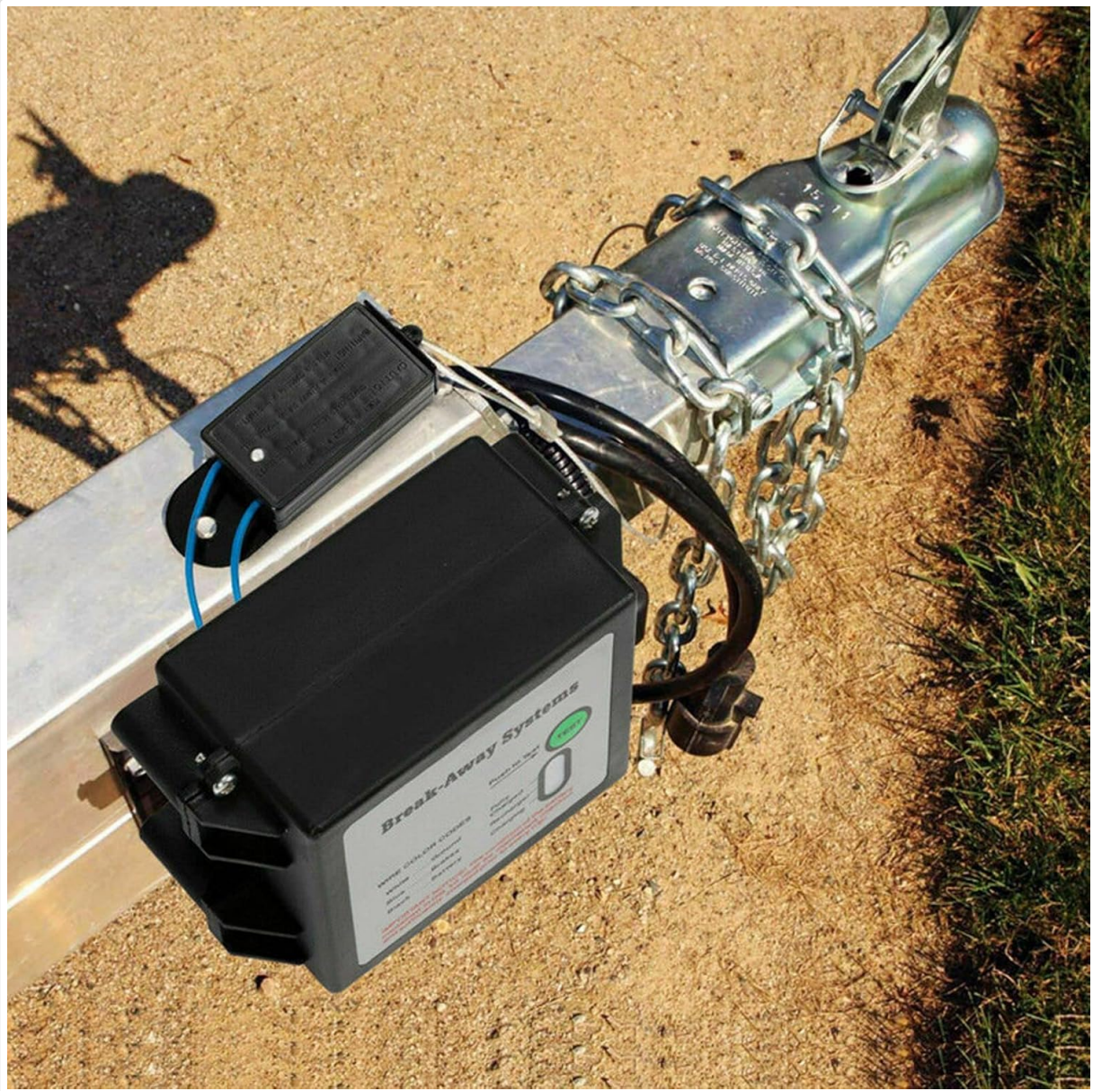
Image: Example of the Tiiyee Breakaway Kit installed on a trailer tongue, showing its connection to the trailer's electrical system.
