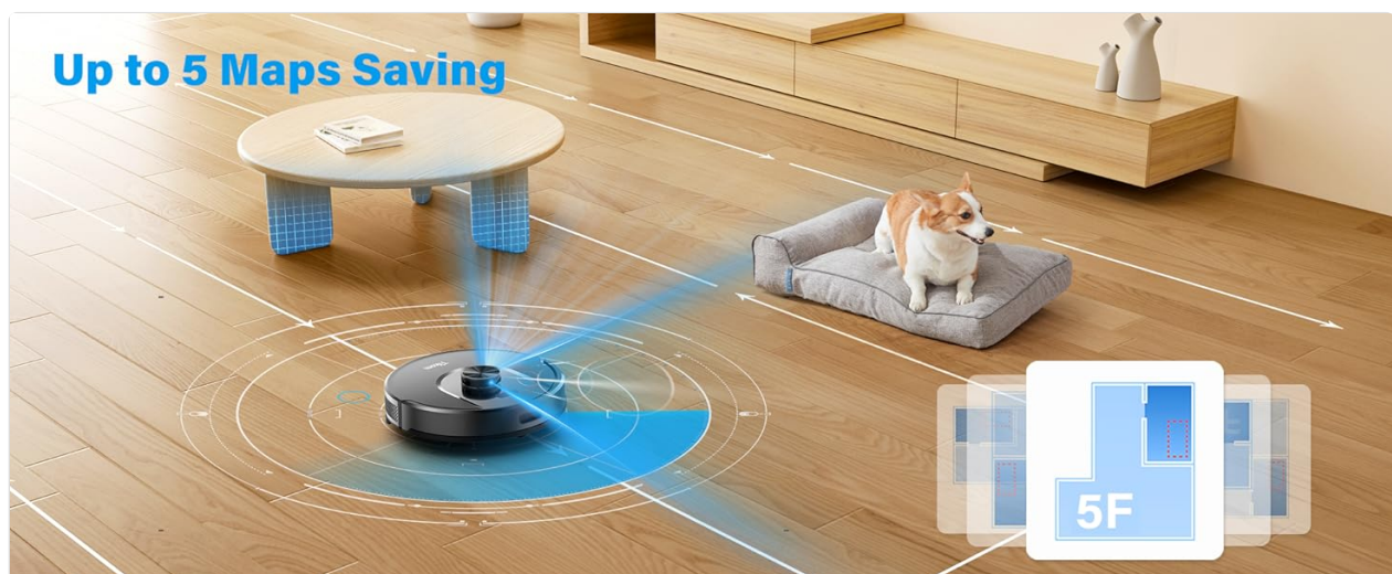
Image 3.1: The robot vacuum utilizing LiDAR navigation to map a room, with an overlay showing the ability to save up to 5 maps for different floors.
