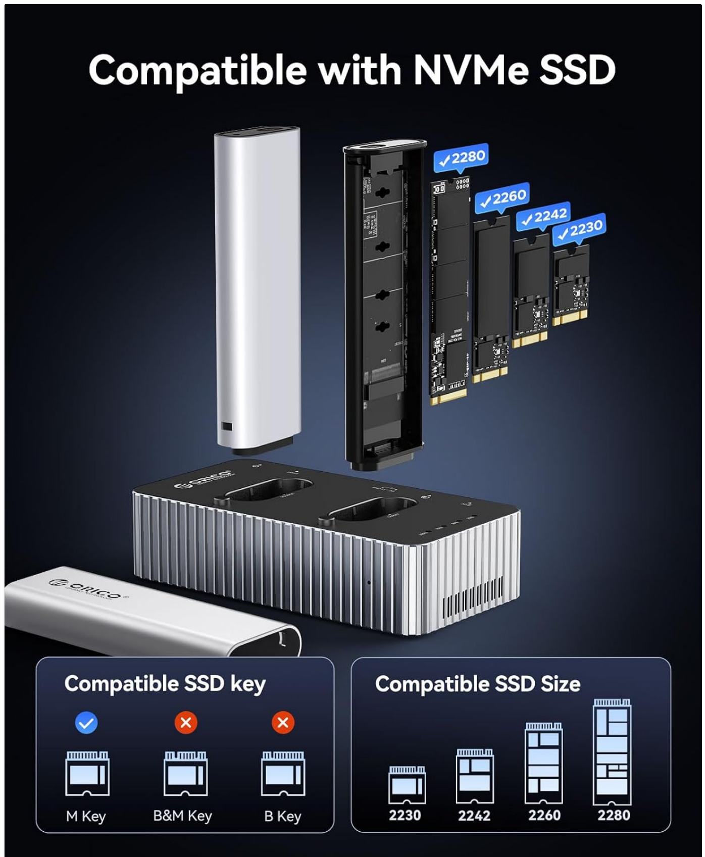
Figure 6.1: SSD Compatibility. This diagram illustrates the supported M-Key NVMe SSDs and various physical sizes (2230, 2242, 2260, 2280) that can be used with the docking station.
