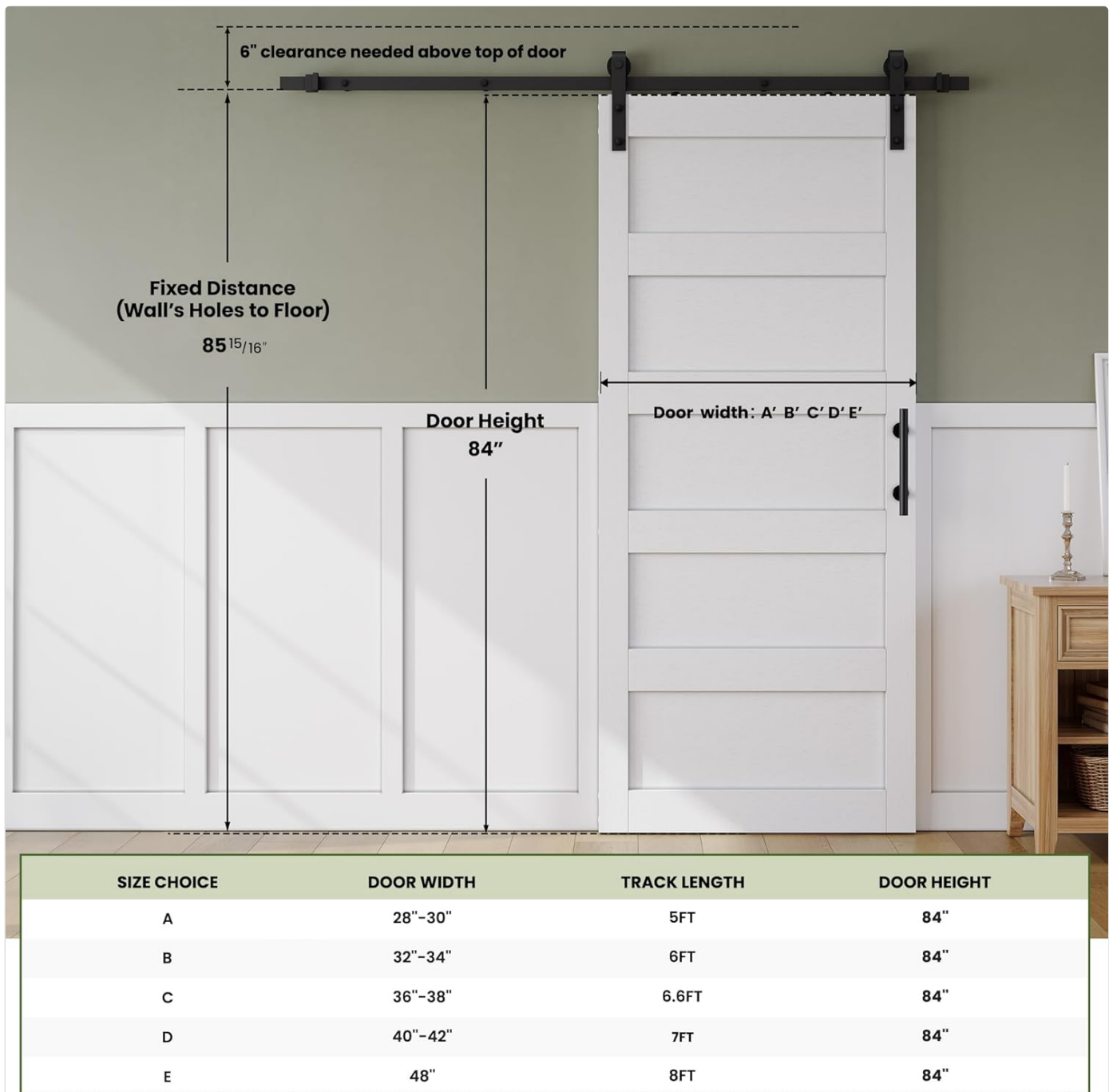
Image: A detailed diagram showing the dimensions of the barn door, the required 6-inch clearance above the door for the track, and a table outlining various door widths and corresponding track lengths.
