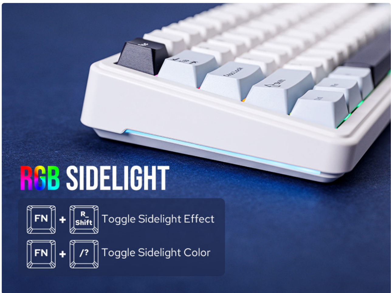
Image 4.2: Close-up of the F65 keyboard's side, highlighting the RGB sidelight and showing key combinations to toggle sidelight effect (FN + Right Shift) and sidelight color (FN + /?).
