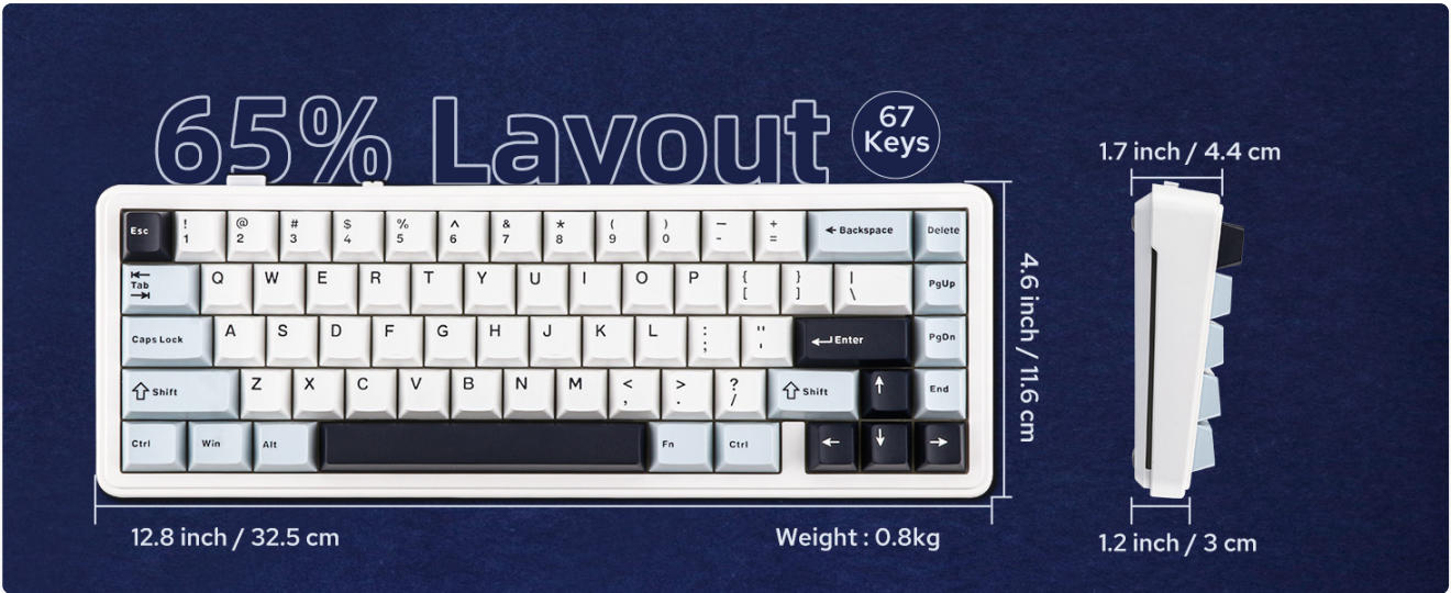
Image 7.1: The F65 keyboard with detailed dimensions: 12.8 inches / 32.5 cm length, 4.6 inches / 11.6 cm width, and height ranging from 1.2 inches / 3 cm to 1.7 inches / 4.4 cm. The weight is indicated as 0.8kg.
