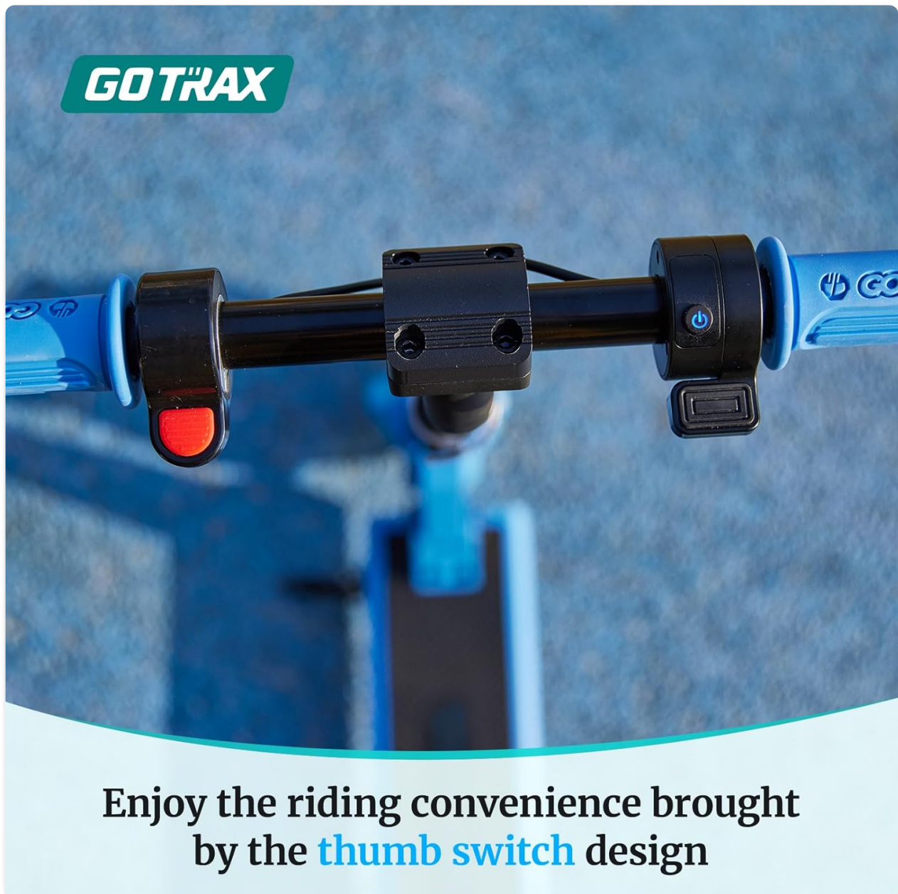
Figure 3: Thumb Button Controls for Acceleration and Braking
