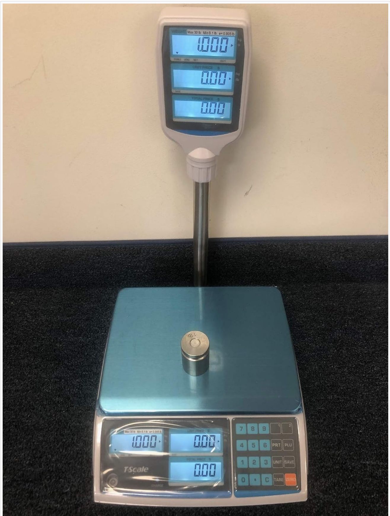
Figure 6.1: The scale displaying a weight of 1.000 lbs on both the operator and pole displays, with the unit price and total price fields showing zeros.
