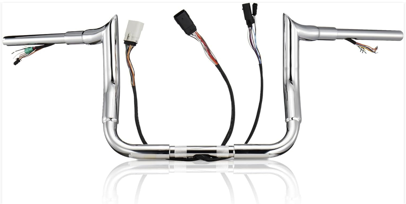
Figure 1.1: MoKitDora Prewired Handlebar, showcasing the chrome finish and integrated wiring for CAN-Bus and TBW systems.
