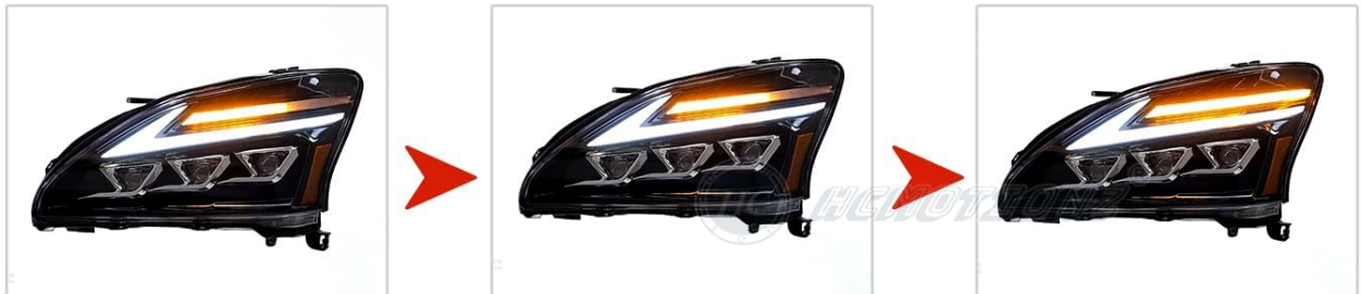
Image 5.2: A three-panel sequence demonstrating the sequential illumination pattern of the LED turn signals.
